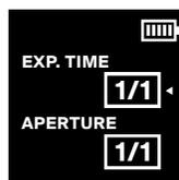
When pressing the thumbwheel for longer than 1 second, a menu is displayed where the increments (step size) of the EXPOSURE TIME, and the APERTURE can be set, respectively. The following increments can be selected:  $\frac{1}{4}$  EV,  $\frac{1}{2}$  EV,  $\frac{1}{3}$  EV, and  $\frac{1}{6}$  EV.
