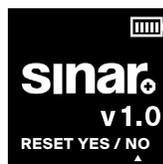
When pressing the thumbwheel for longer than 1 second, the current firmware version is displayed. If necessary, the current settings can be reset to factory default settings by selecting YES and then pressing the thumbwheel briefly.
