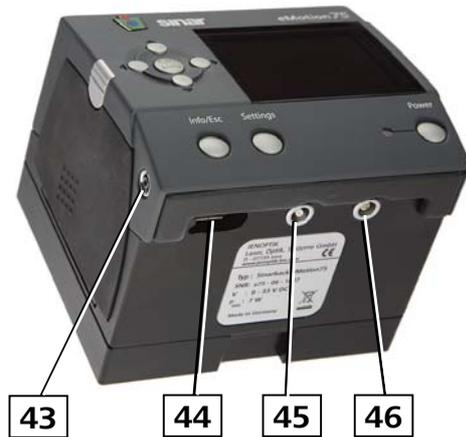
Fig. 24: Connector sockets on Sinarback eMotion 75/54
