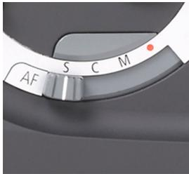
Fig 10 / 1 Operational Area "Focusing Mode"
