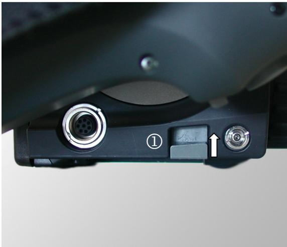
Fig. 5 / 21 Adjustment of the hand grip
