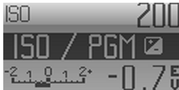
Fig. 11 / 12 Corrected exposure value with light balance
