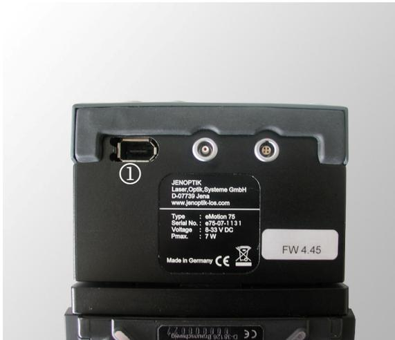
Fig. 5 / 25 IEEE-1394 socket at the back
