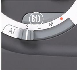
Fig. 8 / 9 Operational area "Focusing Mode"
