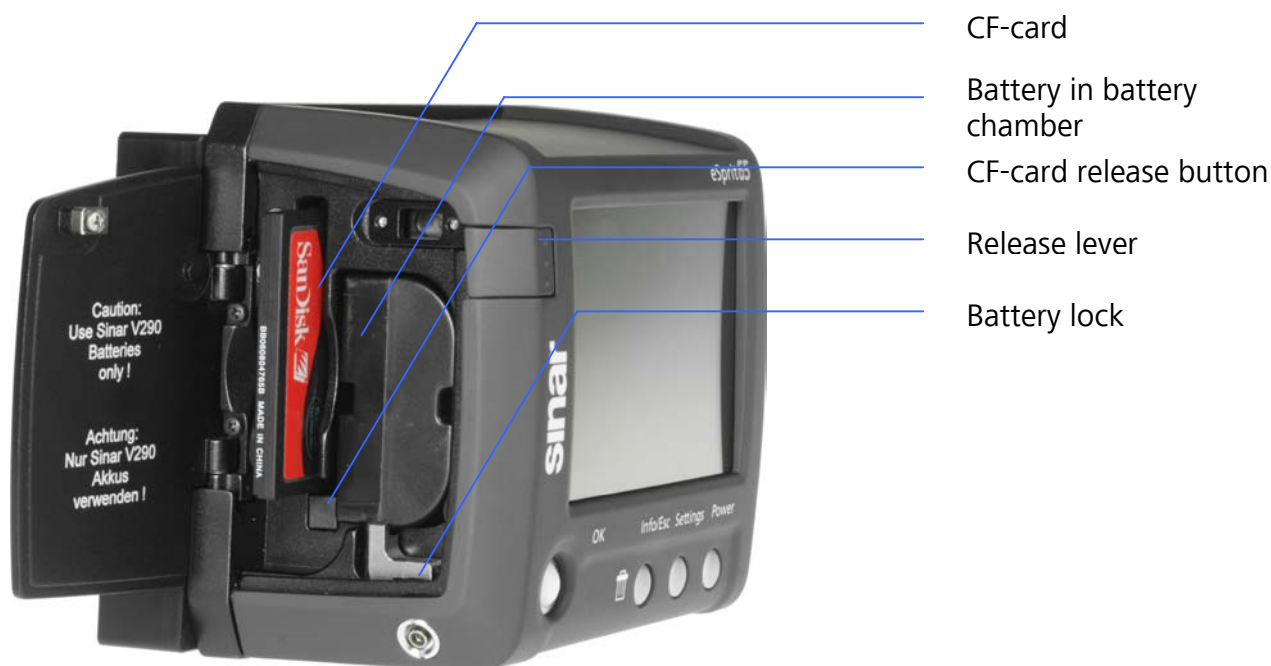
Fig. 5 / 4 Sinarback eSprit 65 LV with open battery compartment
