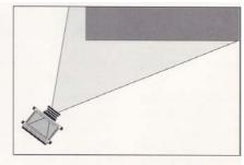
Fig. 30a: When a building is photographed without using the camera movements showing both the front surface and the side of the building, the front facade perspective is bound to converge drastically.
