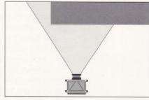
Fig. 30b: When the front of a building is to be shown without converging lines and without using camera movements, the side view of the building disappears. In this case the camera viewpoint is exactly perpendicular to the facade.
