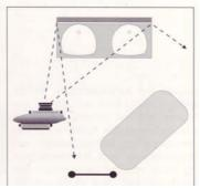
Fig. 31b: Lateral shifts preserve the parallel orientation of lines and the camera is no longer visible on the reflecting surface.
