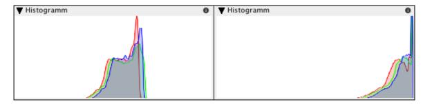
Fig. 44a: Histogram of a correct Shading exposure. Note that neither the left end nor the right end of the curve is clipped.
