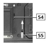
Fig. 26: Advancing the film on a Sinar arTec HB-V
